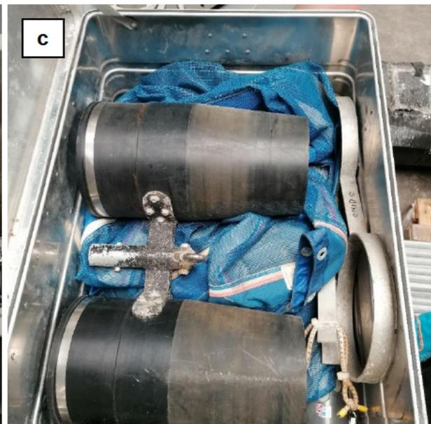
Figure 1: panel a (top) – frame for optical profiler, b (bottom left) – GoFlo bottles, c (bottom right) – miniBongo net with 100 um mesh net.
